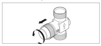
Fig. 2. Remove protection cap
