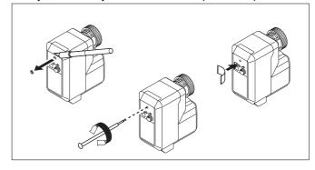
Fig. 10. Adjustment of auxiliary switch S2
