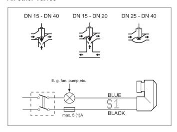
Fig. 13. Electric wiring of auxiliary switch
