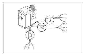
Fig. 9. Auxiliary switch cables
