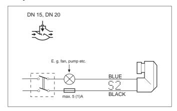
Fig. 12. Electric wiring of auxiliary switch
