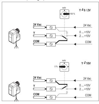
Fig. 6. Connection of input switch
