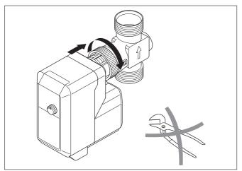
Fig. 3. Mounting the actuator
