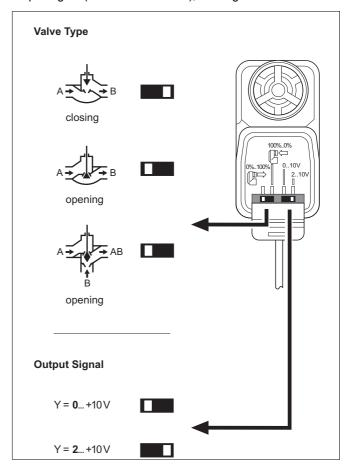
Fig. 4. Selecting valve type and output signal
