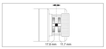
Fig. 8. Movement of the actuator stem
