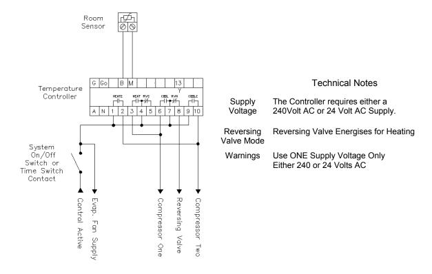
Typical for Compressor Reversing Valve type A/C Units where the R/V energises on Heating
