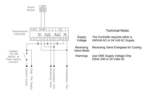
Typical for Compressor Reversing Valve type A/C Units where the R/V energises on Cooling
