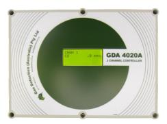
The **GDA 4020** control unit has 2 x 4-20 mA i/p with 3 associated programmable relay alarm levels per sensor. There is an independent fault relay. There are 3 x analog o/p's which can be configured for either channel as 4-20 mA, 0-20 mA, 0-5 V or 0-10 V. The controller has an isolated RS485 o/p which can be configured to drive modbus or an interface to the M2001 mimic panel. All configurations are carried out via the front panel push buttons. The unit requires 24 VDC.
