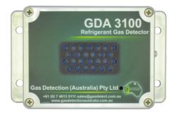
This detector detects generally used **refrigerant** gases (R22, R123, R134a, R404, R407, R410 etc) in the range **0-1000ppm**. Each dectector is calibrated to a specific gas type. It has a configurable analog output, 4-20 mA; 0-20 mA; 0-5 V; 0-10 V.There is also a **volt free relay** which can be user programmed to operate anywhere within the sensor range. The unit is powered from 24 VDC.
