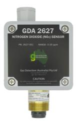
The GDA 2627 **Nitrogen Dioxide** gas **sensor** is a further enhancement of the GDA 2527 **Nitrogen Dioxide** gas **sensor** that allows **AC and DC** operation. It has an **electrochemical** gas sensing unit which is temperature compensated and easily replaceable.
