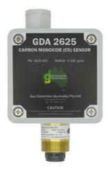
The GDA 2625 **Carbon monoxide** gas **sensor** is a further enhancement of the GDA 2525 **Carbon monoxide** gas **sensor** that allows **AC and DC** operation. It has an **electrochemical** gas sensing unit which is temperature compensated and easily replaceable.
