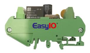
The FR-02 is a relay module which can be mounted on dinrail. It allows 1 x AO coming from a controller to provide floating control via two built-in relays. The modes 1 or 2 are selected by a jumper on the FR-02. Relays rated for 5 million cycles.
