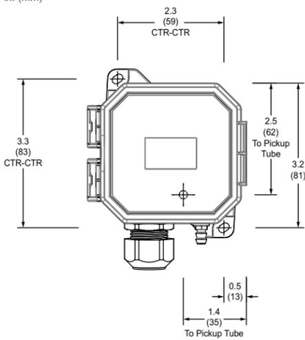
5. For applications using conduit, remove the cable gland nut on the bottom of the unit. Thread a standard 1/2-inch NPT female threaded coupler onto the body of the cable gland. Connect the opposite end of the coupler to the conduit.
