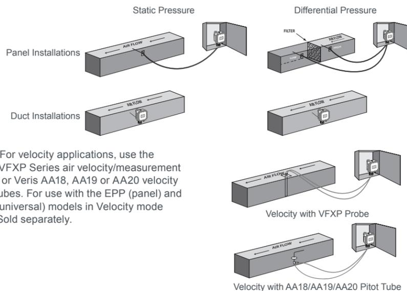
Note: For velocity applications, use the Veris VFXP Series air velocity/measurement probe or Veris AA18, AA19 or AA20 velocity pitot tubes. For use with the EPP (panel) and EPU (universal) models in Velocity mode only. Sold separately.
