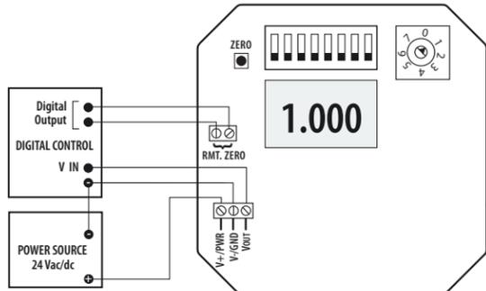
9. Wait five seconds, then press and hold the ZERO pushbutton for two seconds or provide contact closure on the AUX ZERO terminal. This will reset the output and display to zero pressure. For best accuracy, press the ZERO button while both ports are open to atmospheric pressure. To protect the unit from accidental zero, this feature is enabled only when the detected pressure is within about 0.1 in. WC (25 Pa) of factory calibration.
