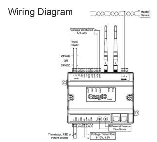
The FW-8V comes with one standard RS485 driver to support BACnet MSTP. The FW-8V also comes with two Ethernet Ports to program the Sedona Application, TCOM, FGP2P, BACnet and for web configurations.
