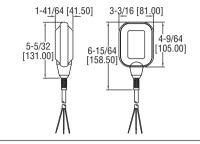
The **SERIES CFS2** Cable Float Switches is a mechanically actuated floating switch intended to activate electrical components, such as pumps, to start and stop automatically. Optional cables are available. Contact factory for cable length options ranging from 10 to 70' (3 to 21 m).
