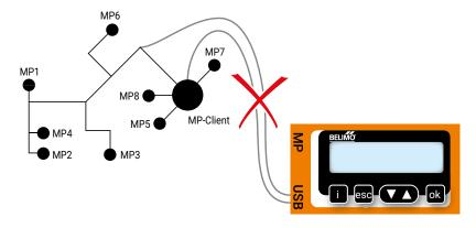
**Solution:** Use service socket on actuator or temporarily disconnect MP connection of MP device from MP-Bus. Connect the ZTH EU to the MP connection.
