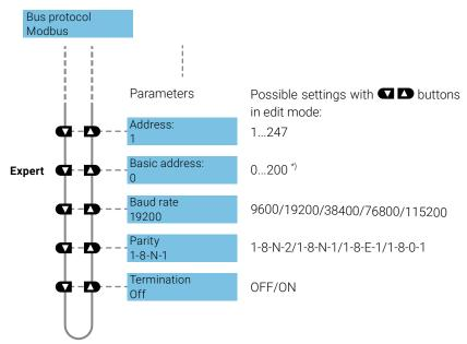
$^{*)}$ The setting of the base address is also taken into account for the BACnet MS/TP address.
