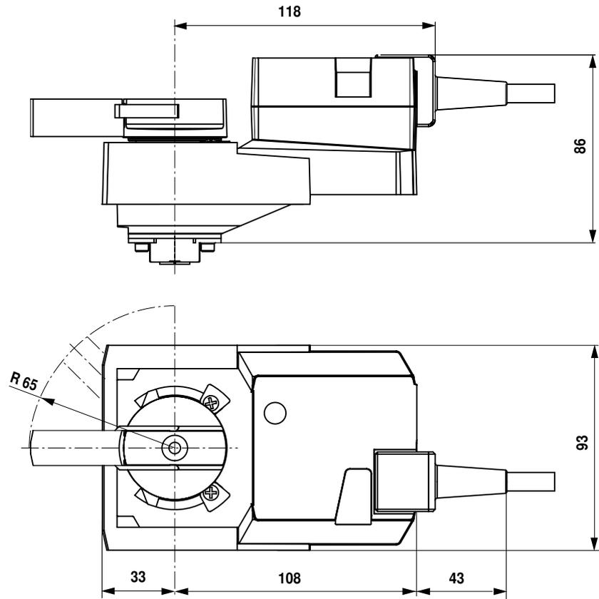
**Rotary actuator for ball valves**
