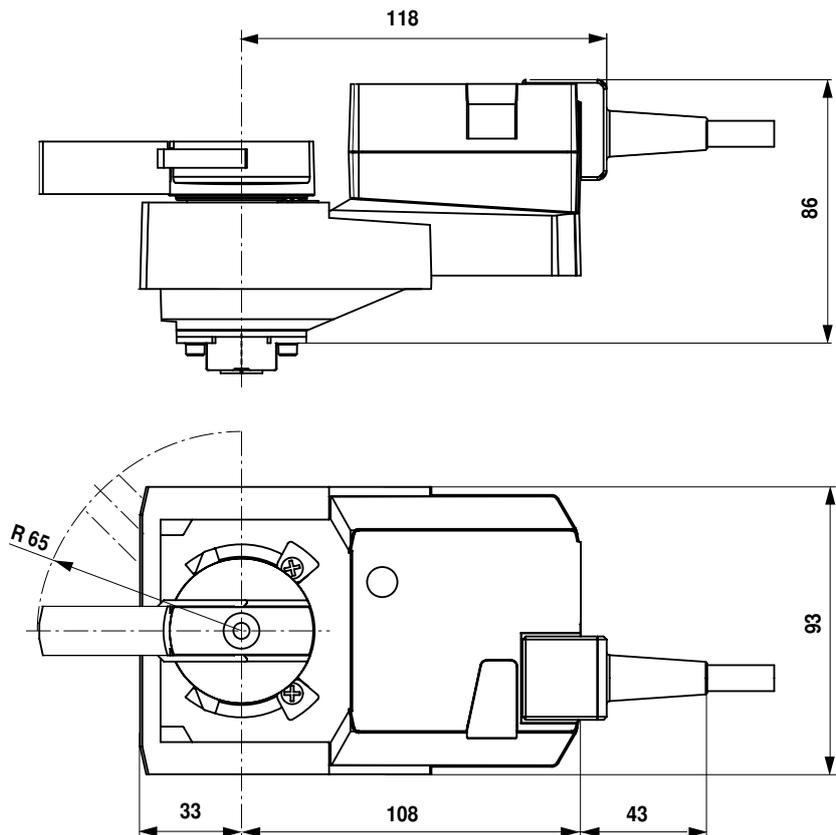
**Rotary actuator for ball valves**
