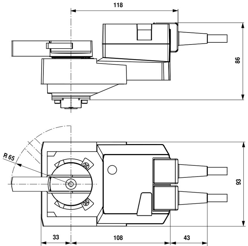
**Rotary actuator for ball valves**
