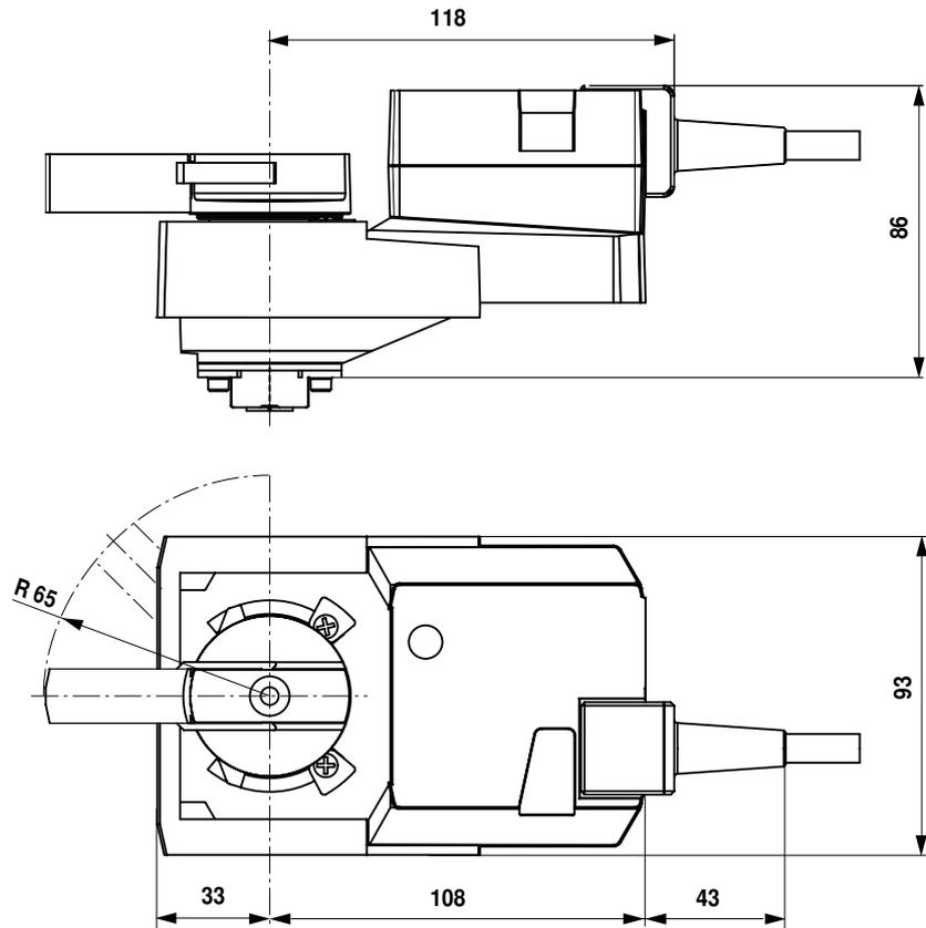
**Rotary actuator for ball valves**
