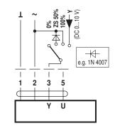
Remote control 0...100% with Minimum limit with positioner SG.. positioner SG..
