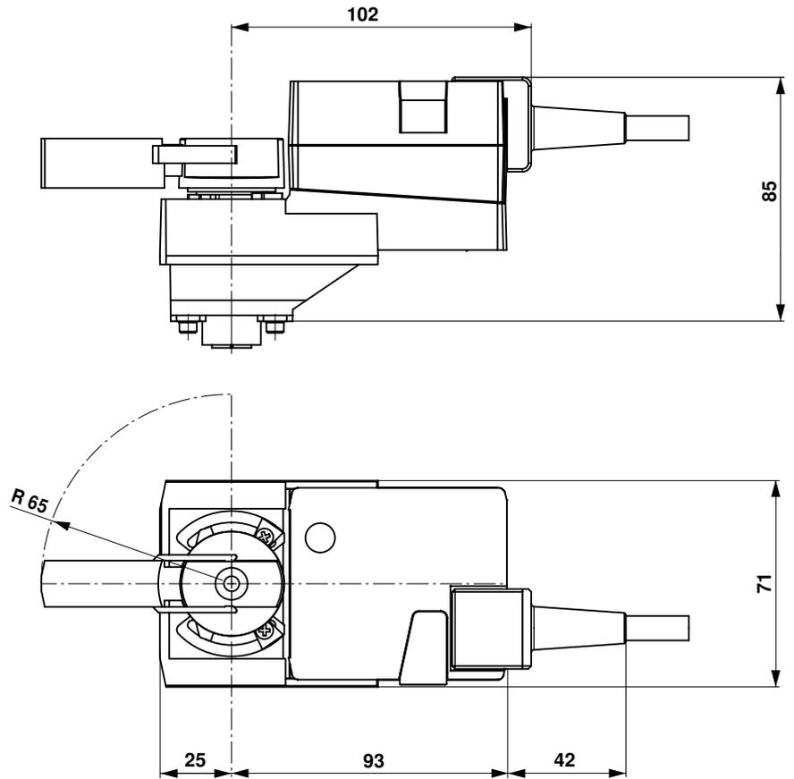
**Rotary actuator for ball valves**
