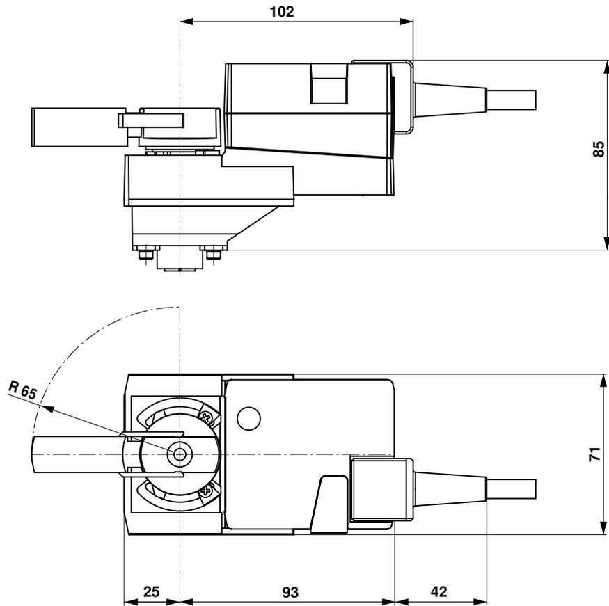
**Rotary actuator for ball valves**
