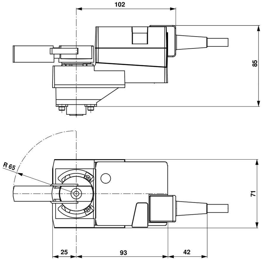
**Rotary actuator for ball valves**
