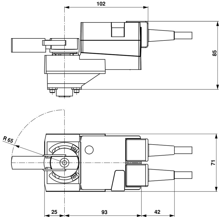
**Rotary actuator for ball valves**
