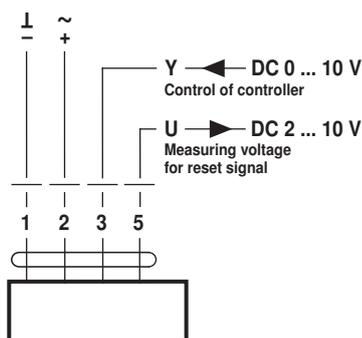
Override control (Frost protection circuit)
