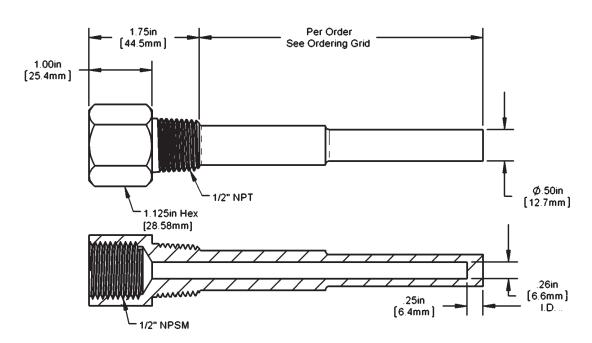
**NPT= National Pipe Taper NPSM=National Pipe Straight Mechanical (not tapered)**
