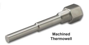
Standard Thermowells available from BAPI include machined 304 stainless steel, 316 stainless steel, brass. These wells are offered in 2", 4" and 8" lengths with 1/2" NPT external and 1/2" NPSM internal. Other lengths and thread diameters are available upon request.
